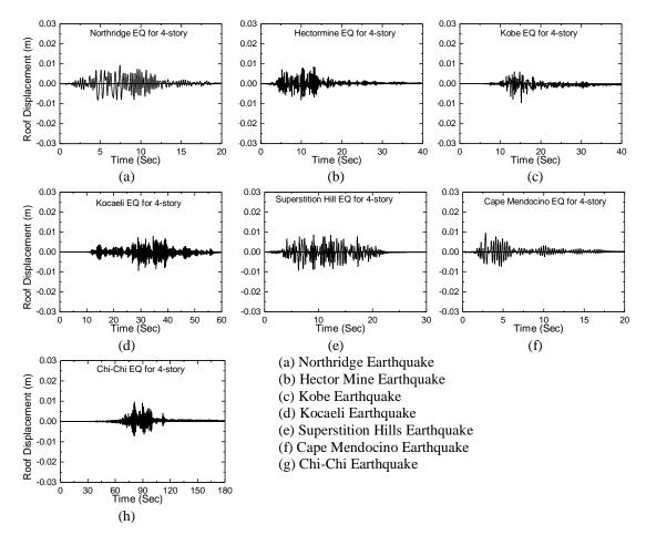
Figure 5. Roof displacements vs. time response of the 4-story frame
