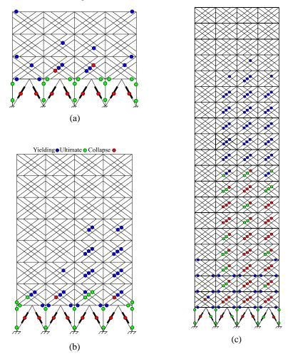
Figure 4. Comparison of hinge mechanism of strengthened frames (a) 4-story, (b) 8-story, (c) 20-story
