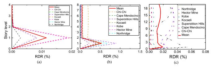
Figure 7. Comparison of residual drift response (RDR) of strengthened frames (a) 4-story, (b) 8-story, (c) 20-story
