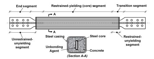
Figure 2: A typical BRB showing different segments along the longitudinal direction and cross-section
