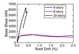
Figure 3: Comparison of capacity curves of strengthened frames
