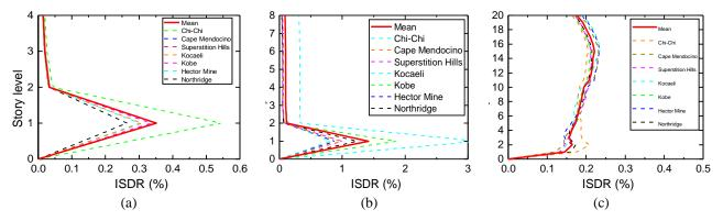
Figure 6. Comparison of inter-story drift response of strengthened OGS frames (a) 4-story, (b) 8-story and (c) 20-story
